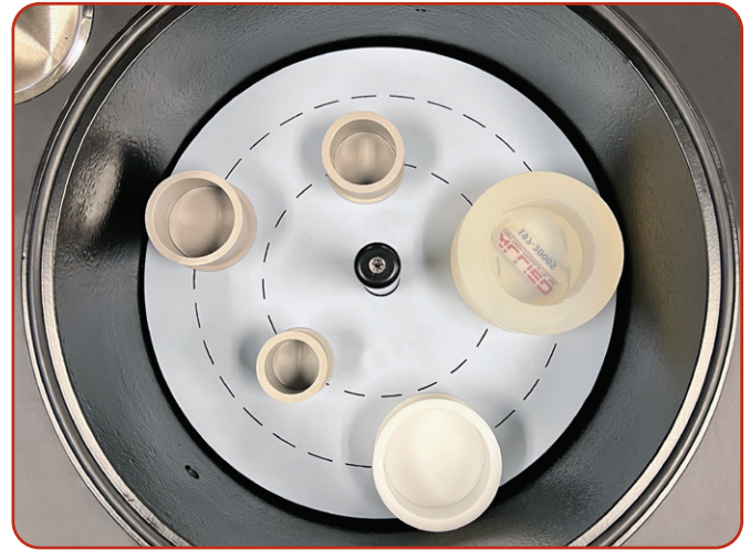
Large 10" (254 mm) diameter chamber (turntable version shown with guide marks for mounting cups)
