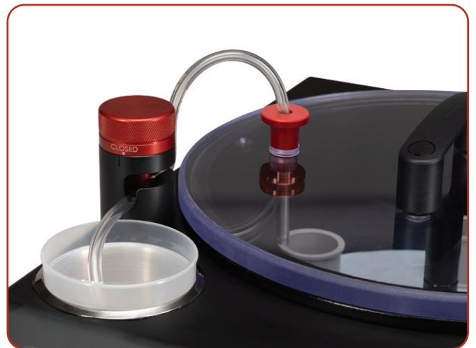
Through-port for optional epoxy fill under vacuum
